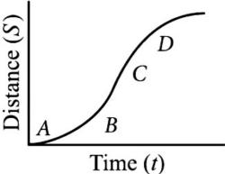
A particle shows distance - time curve as given in this figure. The maximum instantaneous velocity of the particle is around the point (2008)
